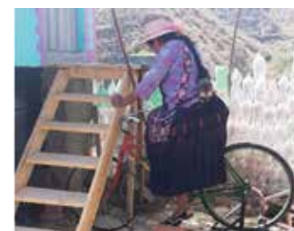
Figure 5. Pedal powered pump prototype. Source: Hábitat para la Humanidad Bolivia, 2021.
